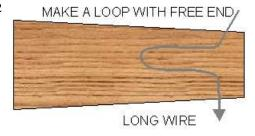
Start wrapping the wire away from the free end. Every 2 or 3 turns, pull the long end tight while you snug the wrappings tight against each other with your fingernails, so each wrap lies next to the previous wrap. When pulling the wraps tight, slide them away from the blade because the taper gets larger in that direction, tightening the wraps.
